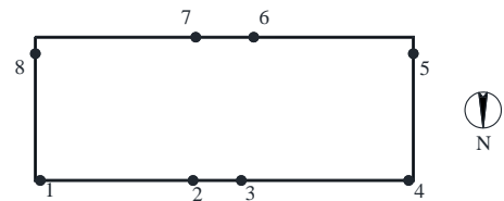
图 13 沉降监测点 (1~8) Fig. 13 Settlement monitoring points (1-8)
