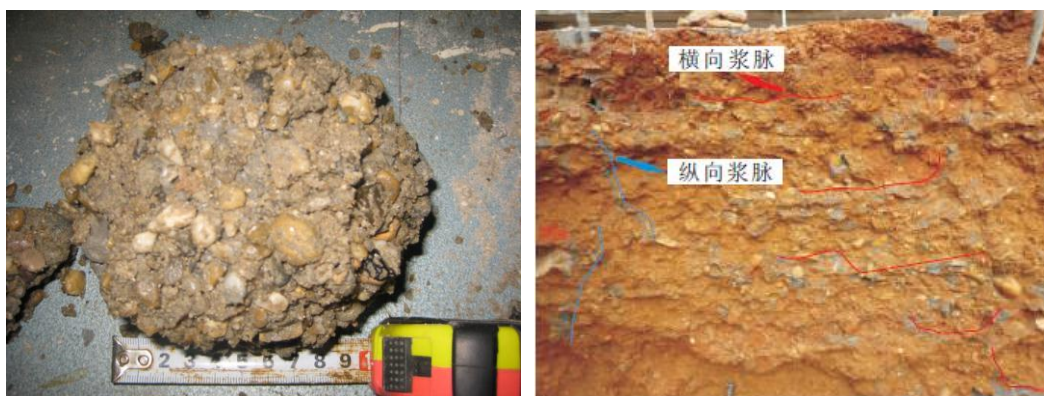
(a) 渗透注浆试验 [22]
