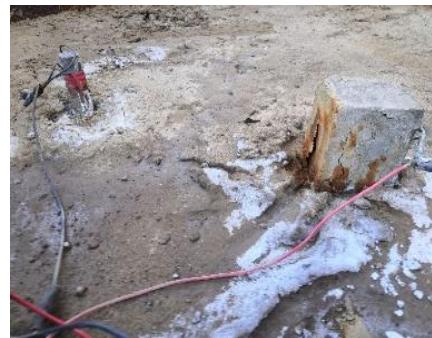
图 5 通电后盐渍土表面析盐现象 Fig. 5 Phenomenon of salt precipitation on the surface of saline soil after electrification
