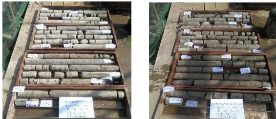
图6 钻孔取芯样 Fig. 6 Core sampling
