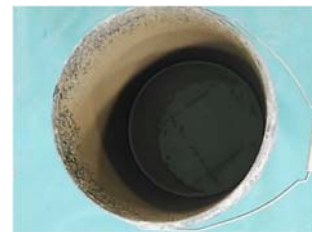
图 1 搅拌均匀后的水泥土试样 Fig. 1 Sample of evenly mixed cemented soil
